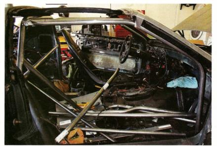
Less than a week later, we received the Chris Alston's Chassisworks weld-in 10-point rollcage we'd ordered, and we started the mockup. Everything from the main hoop and sidebars to the downbars with gussets and mounting plates was included for just \$359. All tubing is constructed with 15/8x0.134-inch-wall mild steel, making it perfectly legal for NHRA and more than adequate for LeMons.
