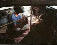
If you don't have experience with a welder, you're going to have to pay someone for the 'cage work. Per LeMons rules, "A poorly built, improperly mounted, or badly engineered rollcage can keep you from racing." Safety is not the place to get sloppy.
