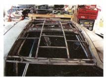
All open and T-top cars require drivers to wear arm restraints. Since none of us are fans, Stroud went ahead and welded in these bars and eventually constructed a roof out of aluminum.
