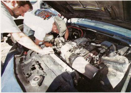
The following morning we added a host of fluids to the engine in hopes of getting a few final laps in, but it just wasn't meant to be. The rod knock was worse than ever, and we even had water spewing out in between the block and driver's side cylinder head. In the end, we placed 95th out of 101 cars and learned that the rod knock video shot by our crew guy Linquist was shown the following Monday on *Good Morning America*. Be sure to drop by chevyhiperformance.com for that video clip.
