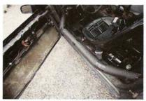
Rather than having the traditional downbar on the driver side, the doors were gutted of glass and everything associated with it to extend the 'cage bar into it.
